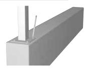
Place the first stand on the base and mark the holes on the plinth or concrete part.
