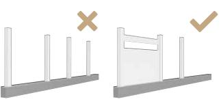
Do not install all the stands: proceed progressively to correct any calculation errors.
