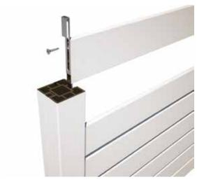
Position the fastening kit at the top section and fasten the screw into the reinforcing core.
