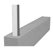
Insert the stand on the cement or in the holes made with the core drill.
