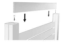
Insert the spacers between each slat into the channel of the post from above.
