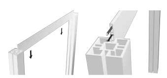
Insert the "Vedo non vedo" slats with 'reinforcing core (20x10 mm cold galvanized) into the groove from the top of the WPC post.
