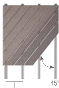
Fig. 2 Decking inclined at 45°
