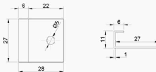
START CLIP (Abmessungen in mm)
