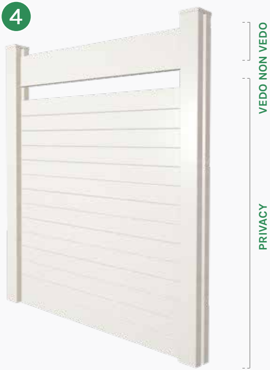
column height H 1650mm, spacing 1520mm 1 VEDO NON VEDO slats + 7 PRIVACY slats with standard 60 mm spacer
