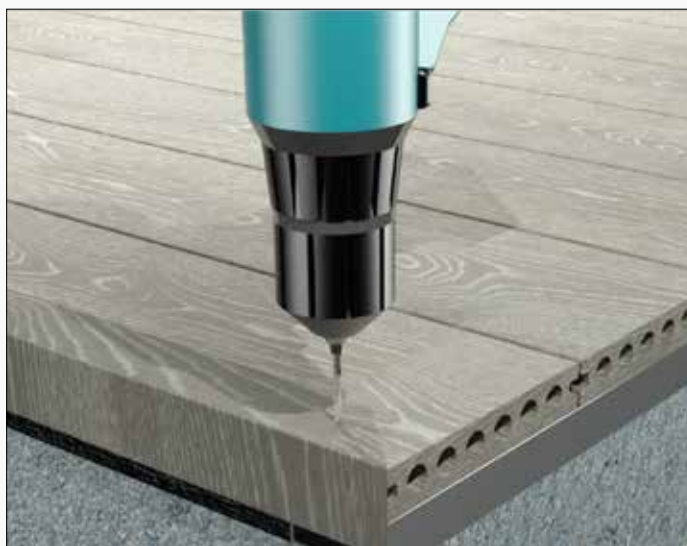
5) Drill with a 3 mm wood bit, to a depth of 25 mm
