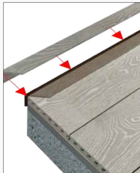
3) Apply the first corner profile (short side) making it match correctly to the slat
