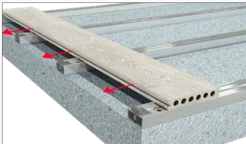
1) Position the slat transversely to the joists and push it until reaching the "start clips"
