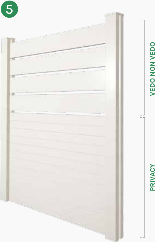
column height H 1850mm, spacing 1520mm 4 VEDO NON VEDO slats + 6 PRIVACY slats with standard 20 mm spacer
